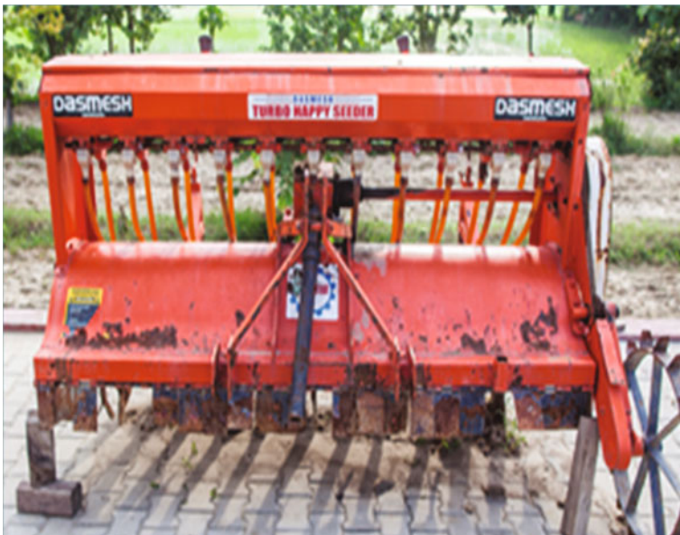
Fig. 4 Picture of Happy Seeder for sowing wheat in the fields
