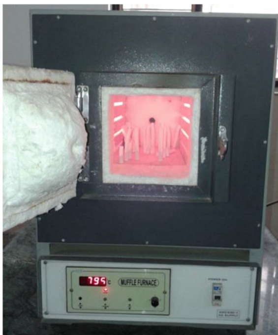
Fig. 2 Chalk pieces heated in muffle furnace at a temperature of 850 °C
