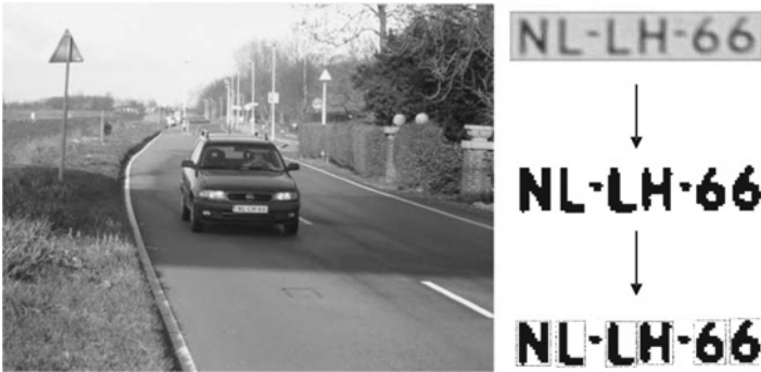
Figure 1.1 Licence plate recognition: a classification problem with noisy measurements.
