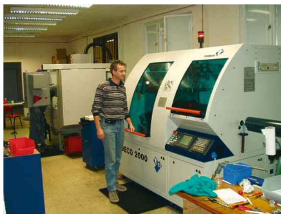
Fig. 1.1. Advanced CNC milling machines are capable of shaping many different BOI designs with defined properties from a single bar of massive titanium
