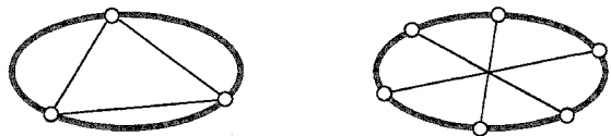
Fig. 4. Potential coplanar configurations for measuring the in-plane V_{xx}, V_{xz} and V_{zz} simultaneously: triangle edges (left) or spokes (right).
