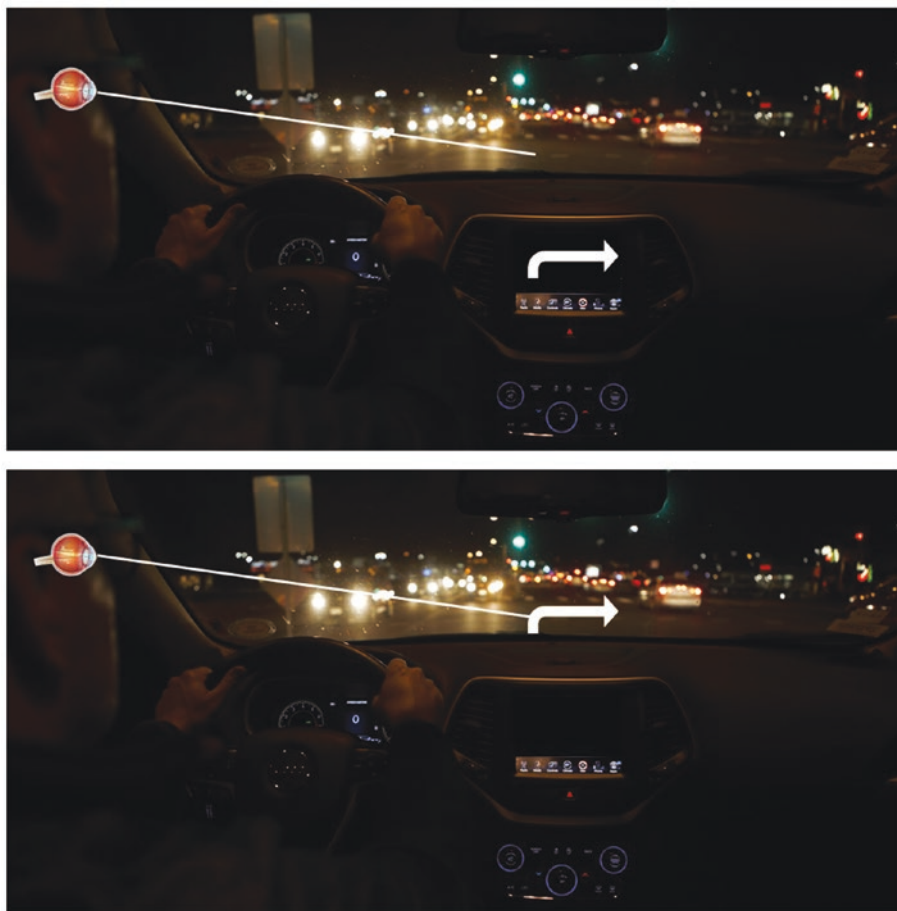
Figure 1-6. Dashboard display challenge. Most design elements on dashboard displays will be unreadable by drivers focusing on the traffic ahead unless they are projected onto the windshield. ix
