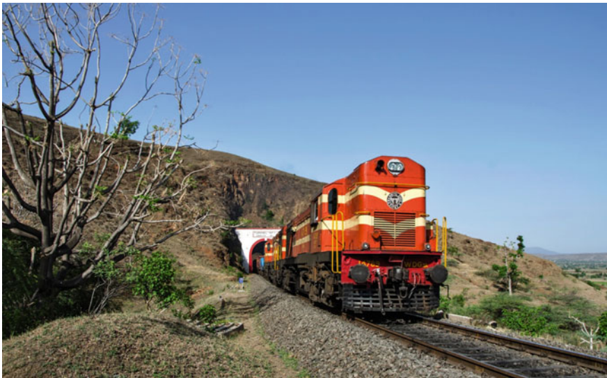
Fig. 4 WDM3A class locomotives with high-adhesion bogies for heavy freight operations
