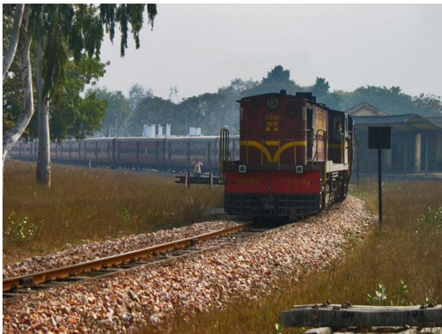
Fig. 2 A DLW manufactured YDM4 meter-gauge diesel of the ALCO design
