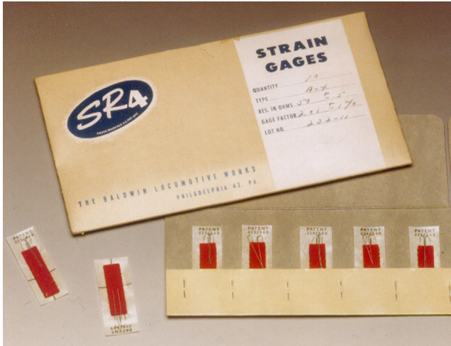
Fig. 1.5 One of the first strain gage packages as sold by Baldwin in 1941
