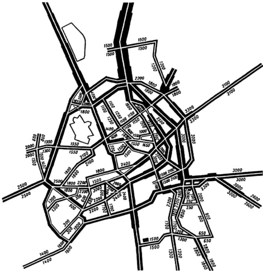
Fig. 1.7 The cartogram of the average daily traffic flow in the city [Source Klinkovshteyn (1975)]
