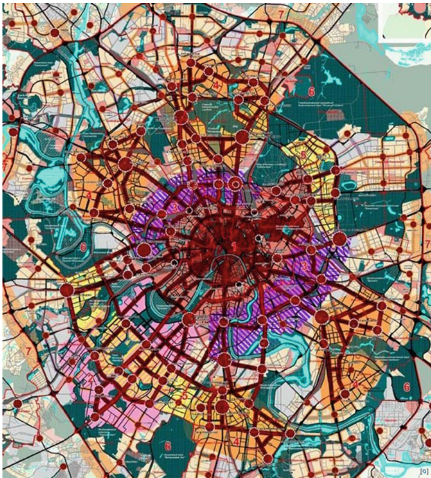
Fig. 1.9 General plan of Moscow during the mayorship of Yuri Luzhkov (1990–2005). The emphasis on the reconstruction of road junctions is clearly visible ( large and small circles )
