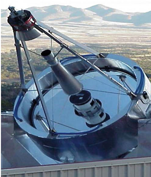
Fig. F6 Two-meter automatic spectroscopic telescope at the Fairborn Observatory
