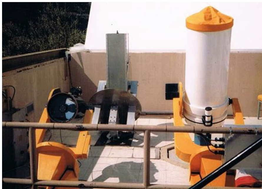
Fig. F4 The original three robotic telescopes at the APT Service on Mt. Hopkins. Left to right: the Fairborn-10, the Phoenix-10, and the Vanderbilt-16
