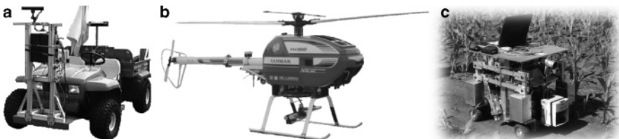
Figure 1.5 Innovative field vehicles: (a) utility platform; (b) spraying helicopter; (c) scouting robot (courtesy of Yoshisada Nagasaka)
