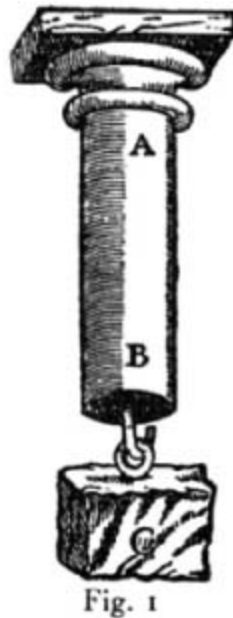
Figure 1.1. Longitudinal pull test (Galileo, Discorsi, 1st day [GAL 38a])
