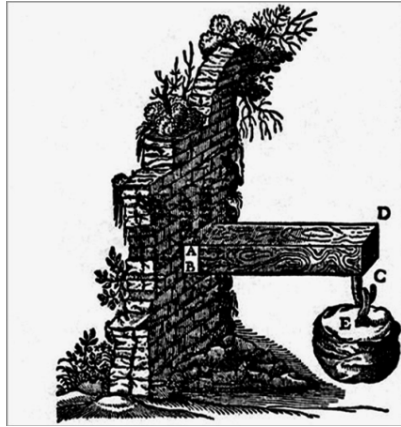
Figure 1.2. Prism subjected to the transverse application of a weight (Galileo, Discorsi , 2nd day)
