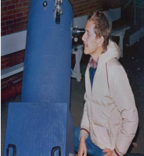
Fig. 1.2 Greg Boles of Topeka, Kansas, is using a 1980s Coulter Optical “Blue” tube “rocker box” style 13.1-in. f/4.5 Dobsonian to observe the heavens with (Image credit: Rick Schmidt)
