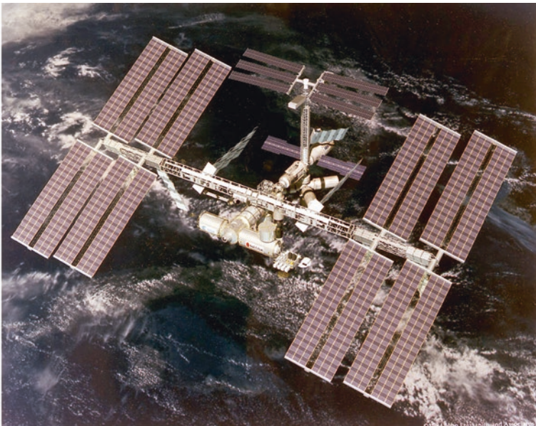
In this image of the completed ISS the American segment, with the European and Japanese laboratories, is shown the foreground, this time with the planned Russian segment in the background.
