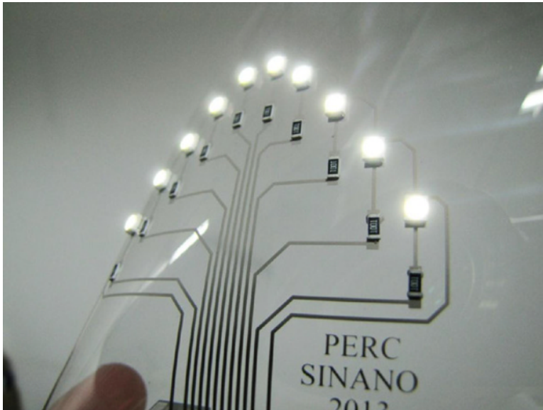
Figure 1.7 Flexible circuits on transparent plastic film made by inkjet printing of nanosilver ink
