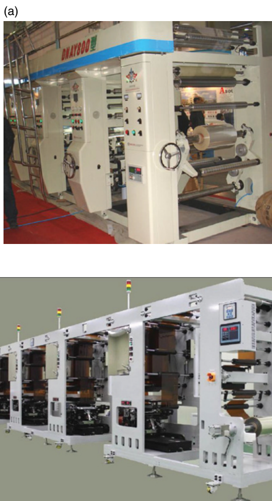
Figure 1.2 Comparison of (a) conventional paper media printer; and (b) electronics printer. (Courtesy of iPEN Co. Ltd.)
