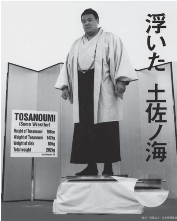
Figure 1.4 Application of free levitation by means of the permanent currents in a superconductor. The Sumo wrestler (including the plate at the bottom) weighs 202 kg.
