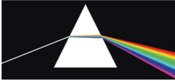
FIG. 1.3 When white light passes through a glass prism, a spectrum of colors is produced (Image by the author)
