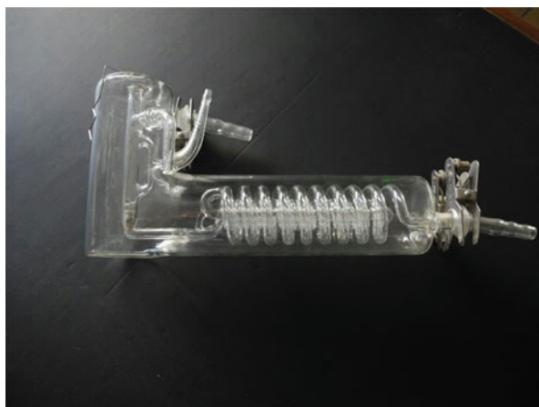
Fig. 2 Organ bath used in the author's laboratory (PH) in the 1980s
