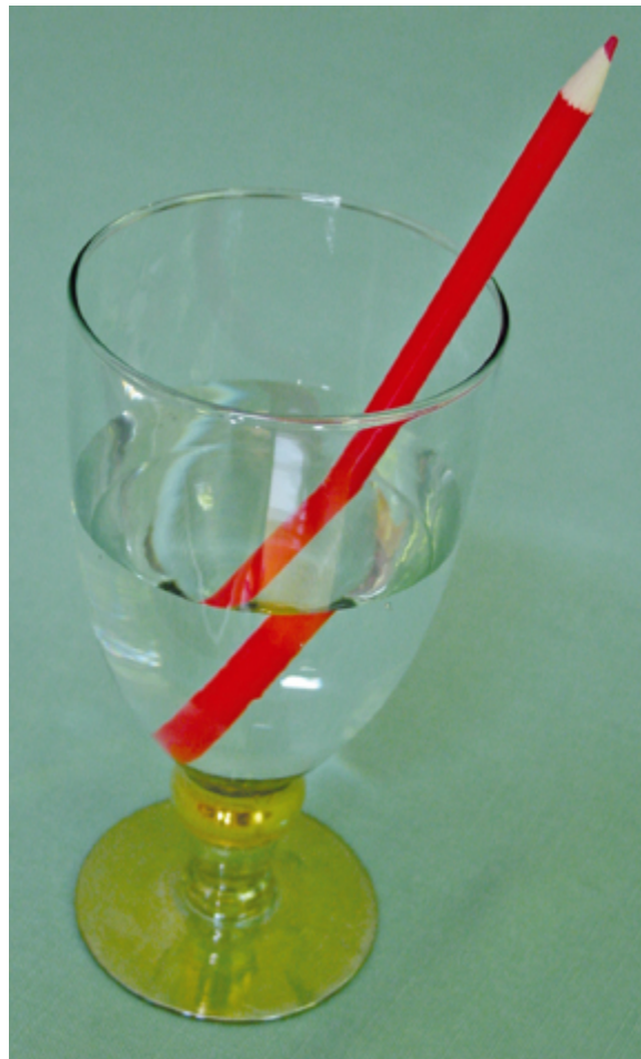
FIGURE 1.8 The apparent bending of the pencil and the double image is due to refraction effects.
