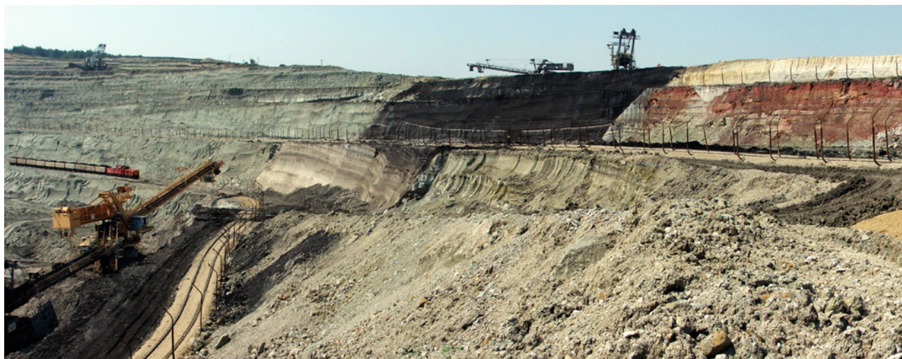
Fig. 2.9 Open pit mine Družba in the Neogene Sokolov basin located in the Ohře/Eger graben. Coal seam outcropping along boundary normal fault. In the footwall ( right side ) weathered metamorphic rock of
