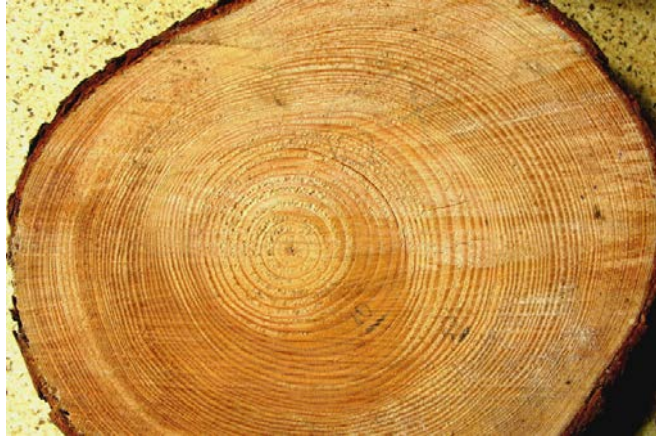
Figure 1.1. Cross-section of softwood (in this case Pinus Silvestris L.)
