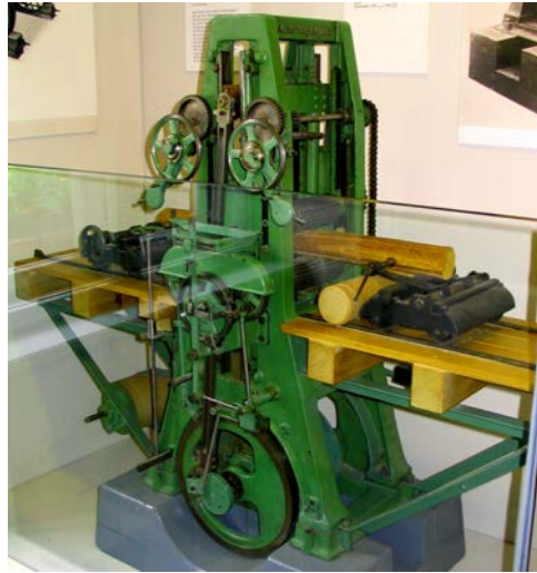
Figure 1.8. Construction of the frame sawing machine (miniature in the Holztechnisches Museum Rosenheim, Germany)
