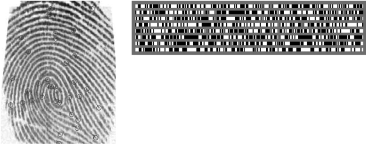
Figure 1.6. Minutiae extracted from a fingerprint image (on the left) and binary code of the iris (on the right)
