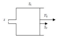
EXAMPLE 1.1 (<u>Figure 1.2</u>). We consider a cylinder inside of which a piston moves at velocity  $V_0$ . Calculate the debit on entry of an incompressible fluid.
