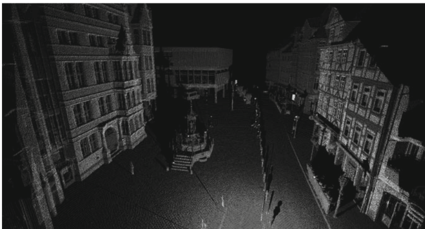
Fig. 1.2 Visualization of a 3D point cloud acquired with a terrestrial laser scanner and colored with respect to the respective radiometric data
