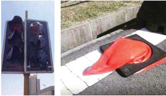
Picture 1.1 Kuwait City (60 C, July 3, 2016), the heat melted the rubber shades.
