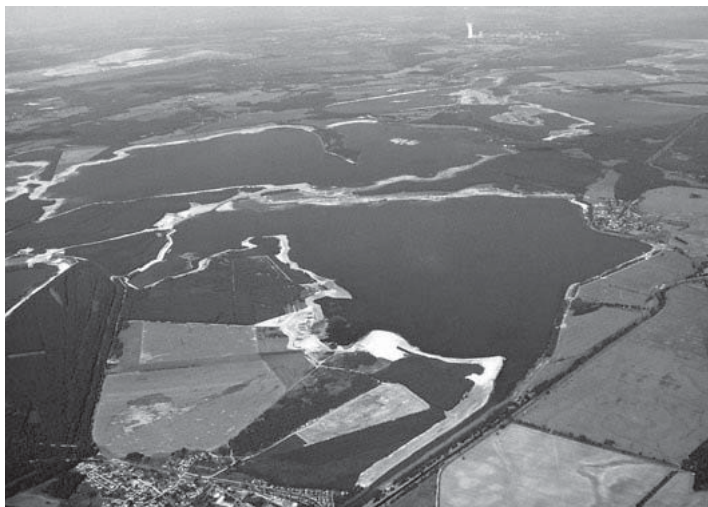
Fig. 2: In Lusatia (Germany) 21 former open cast pits from lignite mining will be flooded by 2017, forming the Lusatian Lake District (photo: Radke/LMBV)
