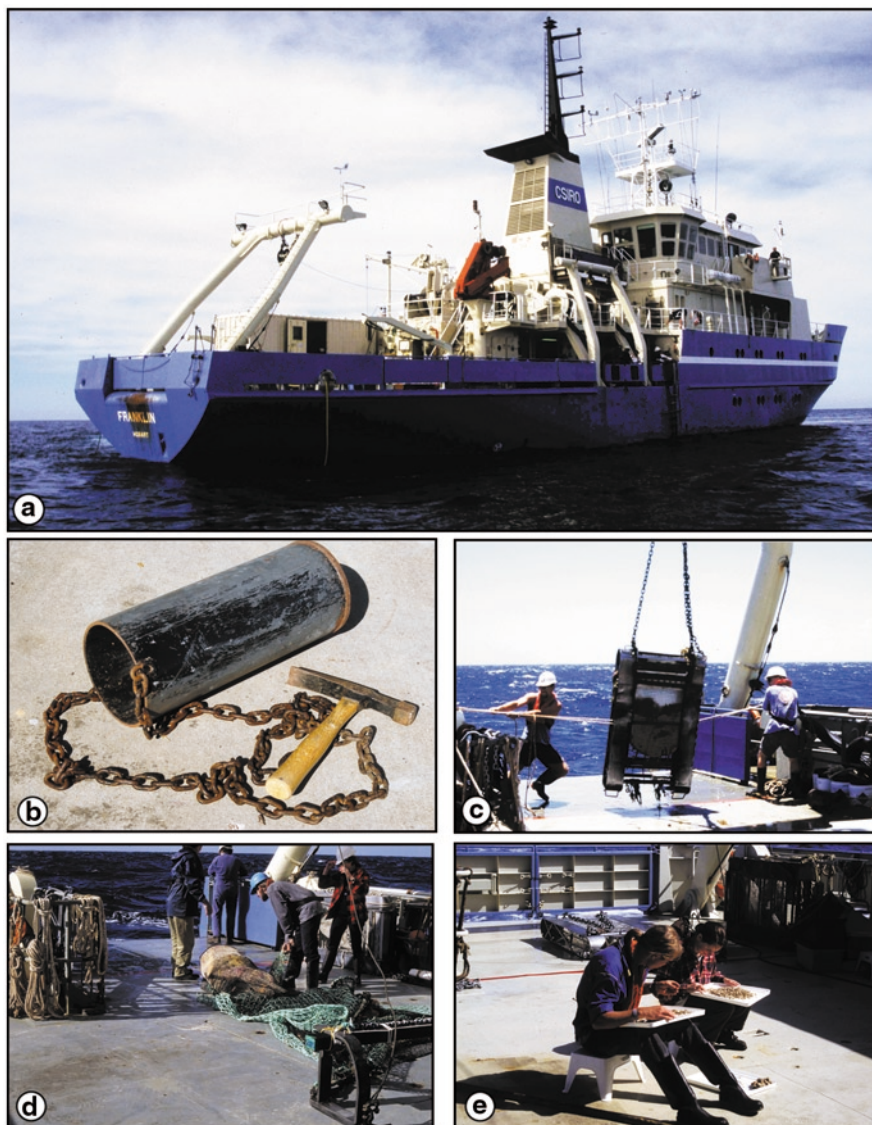
Fig. 1.5 (a) RV Franklin , the platform used to collect most of the samples and other marine information used in this book, (b) the pipe dredge (Bleys Dredge) used to collect most of the bottom sediment samples; hammer is 15 cm long, (c) the epibenthic sled being retrieved after sampling; the bag in the center is half full of sediment, (d) the material, seafloor biota, and sediment recovered by a beam trawl, (e) sediment being analyzed on the stern deck of RV Franklin . (Paul Gammon and Kirsty Brown)
