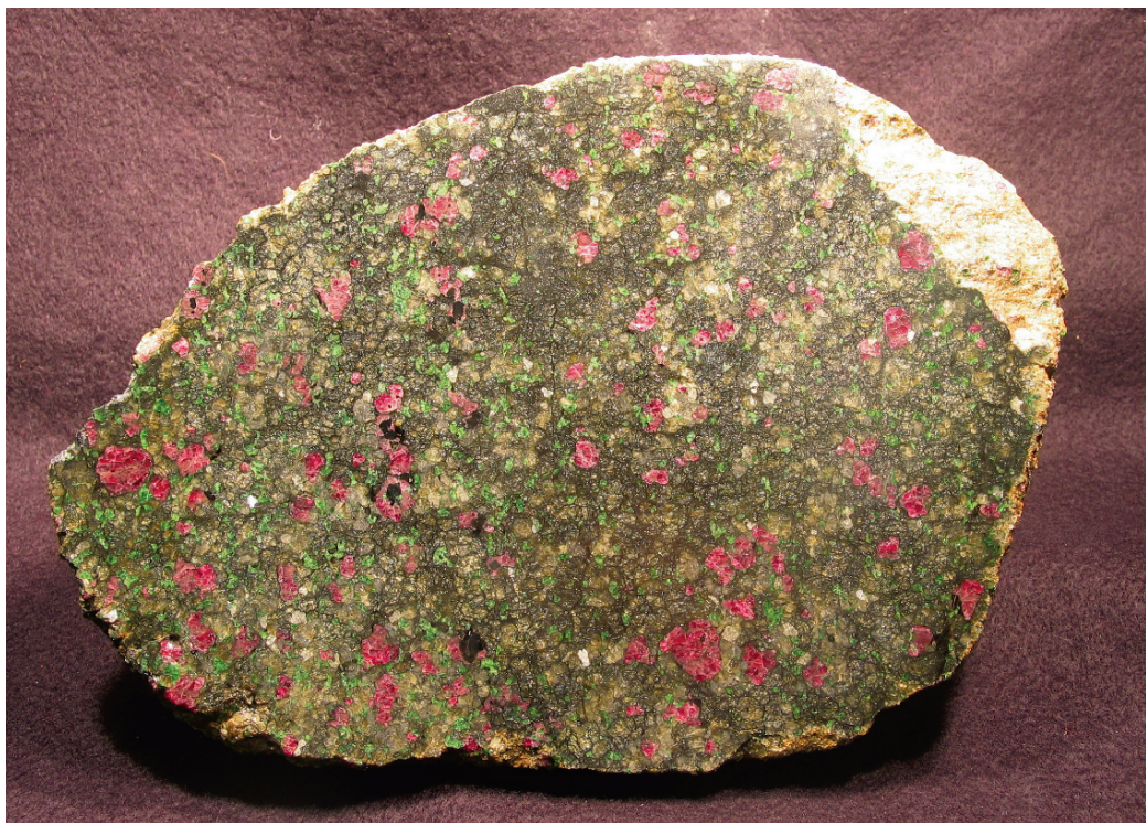
1-04: A piece of the lithospheric mantle: peridotite xenolith from the Bultfontein mine, Kimberley, South Africa (Ø: ~30 cm), which consists mainly of olivine (dark green), garnet (purplish-red), Cr-diopside (bright green), and orthopyroxene (light brown).
