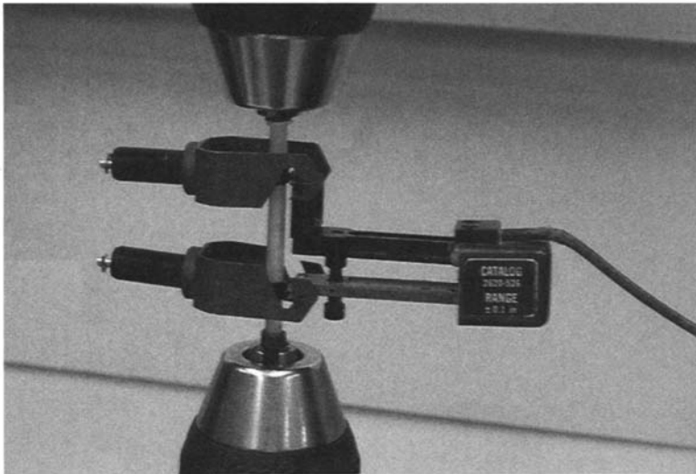
Fig. 2. Tension test setup for wheat/barley specimens. Shown are the load frame jaws, the end grips, the heat shrink collars, and the extensometer.
