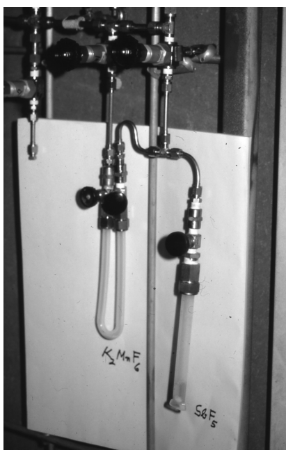
FIGURE 1.1 The original apparatus used by Christie in 1986 for the first chemical synthesis of F 2 . (For a color version of the figure, please see color plates.)
