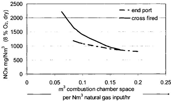
Figure 3. NO<sub>x</sub> emission levels in container glass industry for regenerative furnaces, depending on specific combustion space volume, curves are derived as best fit from many data.
