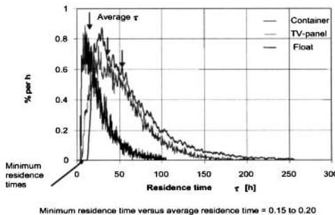
Figure 5. Typical residence time distributions for the melt in different glass melting tanks for float glass, TV panel glass and soda-lime-silica container glass production.
