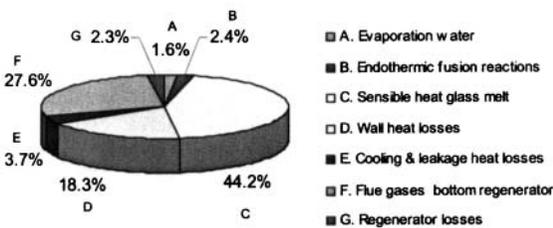
Figure 2. Energy consumption and distribution of energy (losses) in an energy efficient container glass furnace (top 10% in the benchmark pool).
