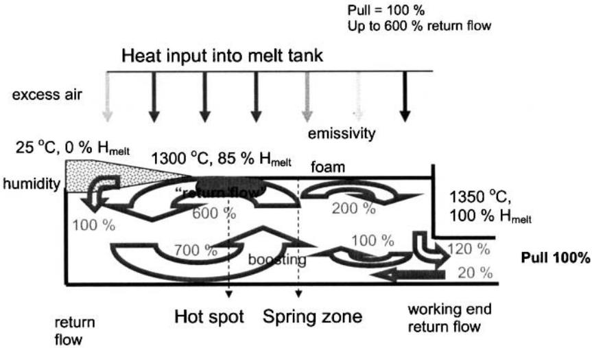
Figure 4. Scheme of main flow patterns in glass melting tank for continuous glass production. The “return flow” from spring zone/hot spot to batch blanket can be more than 6 times the pull. Batch absorbs within about 1 hour, 80-90% of the total net heat input in the melting process.
