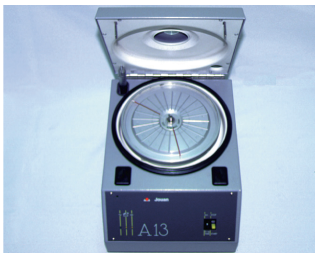
Figure 1.5 Representative microhematocrit centrifuge. The head and motor are designed to spin the tubes at very high speeds to achieve maximal erythrocyte packing.
