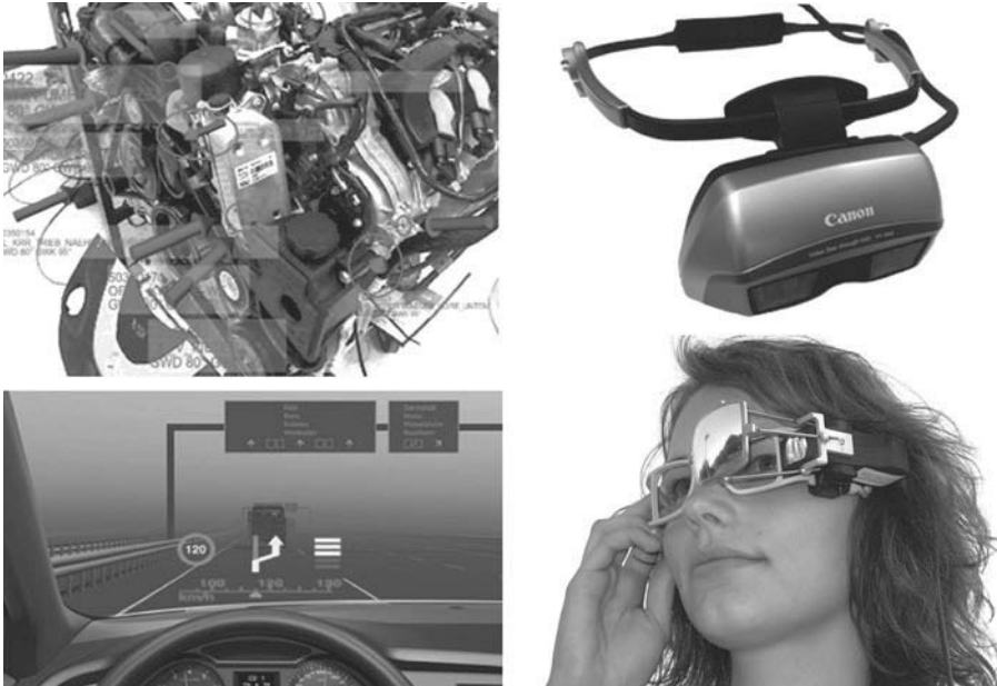
Fig. 5 Sample display devices and AR applications: AR-system for vehicle assembly (top left, source: Brose), video-see-through HMD (top right, source: Canon), automotive head-up display (lower left, source: AUDI) and optical-see-through glasses (lower right, source: Zeiss)
