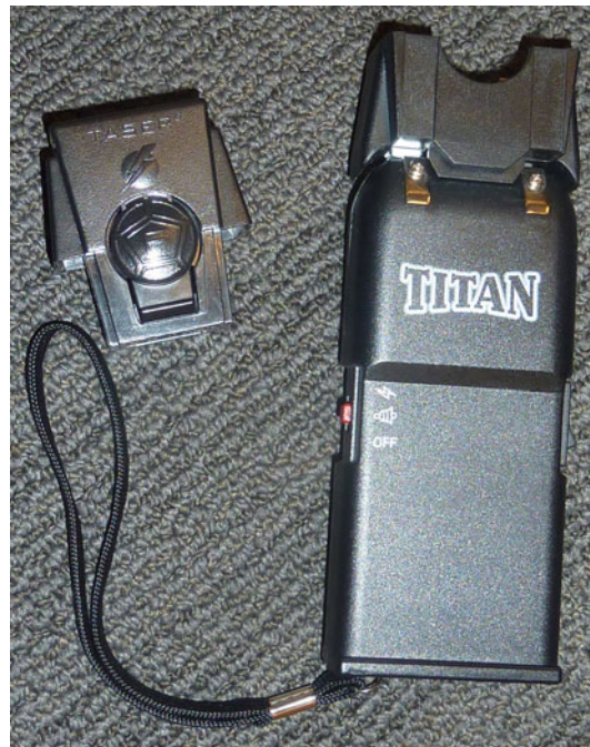
Fig. 1.4 The Titan Taser shown with a genuine TASER device cartridge. This CEW was designed to take advantage of currently available CEW cartridges (Reproduced with express permission of TASER International, Inc., Scottsdale, AZ)
