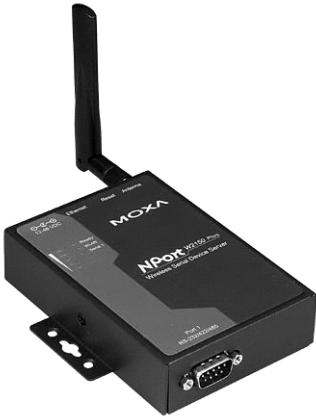
Figure 1-4 Moxa Technologies NPort W2150 Wireless 802.11g to Serial adapter (Courtesy Moxa Technologies, used with permission)
