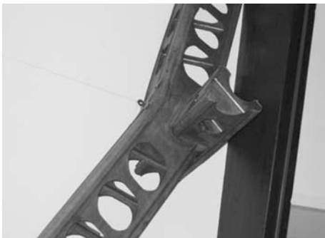
Figure 2.3 A junction between three-dimensional airship girders made from glued wood (Schütte-Lanz, ca. 1915).
