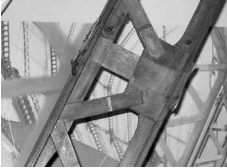
Figure 2.2 The girder of a rigid airship made from glued asp wood (Schütte-Lanz, ca. 1915).
