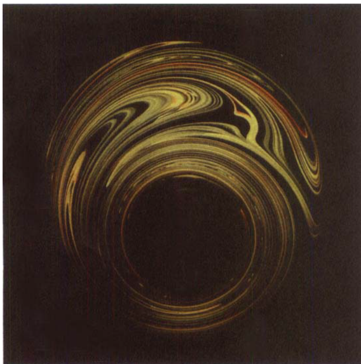
Color Plate 11 Lagrangian chaotic mixing of dye in a fluid between two oscillating cylinders. (Courtesy of Professor J. M. Ottino, Northwestern University, Evanston, Illinois.)
