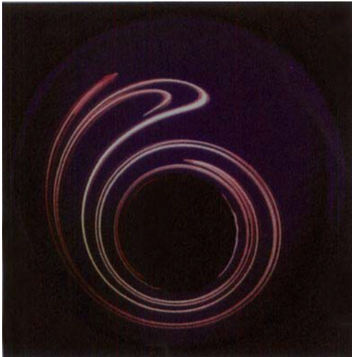
Color Plate 10 Lagrangian chaotic mixing of dye in a fluid between two oscillating cylinders. (Courtesy of Professor J. M. Ottino, Northwestern University, Evanston, Illinois.)
