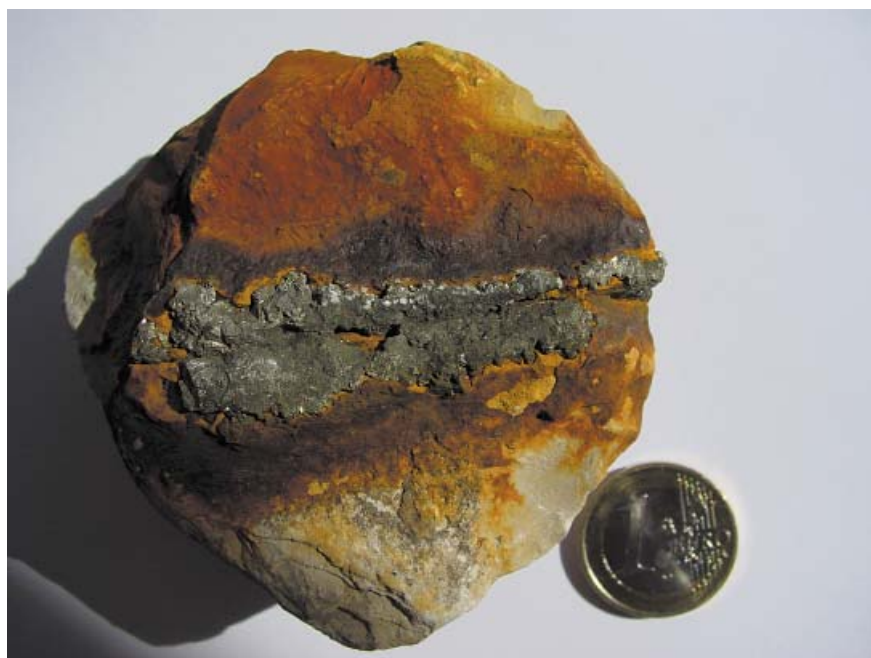
Plate 15.II Iron oxide formation by atmospheric weathering of a pyrite vein in a limestone (photo courtesy, Ph. Jaesche).
