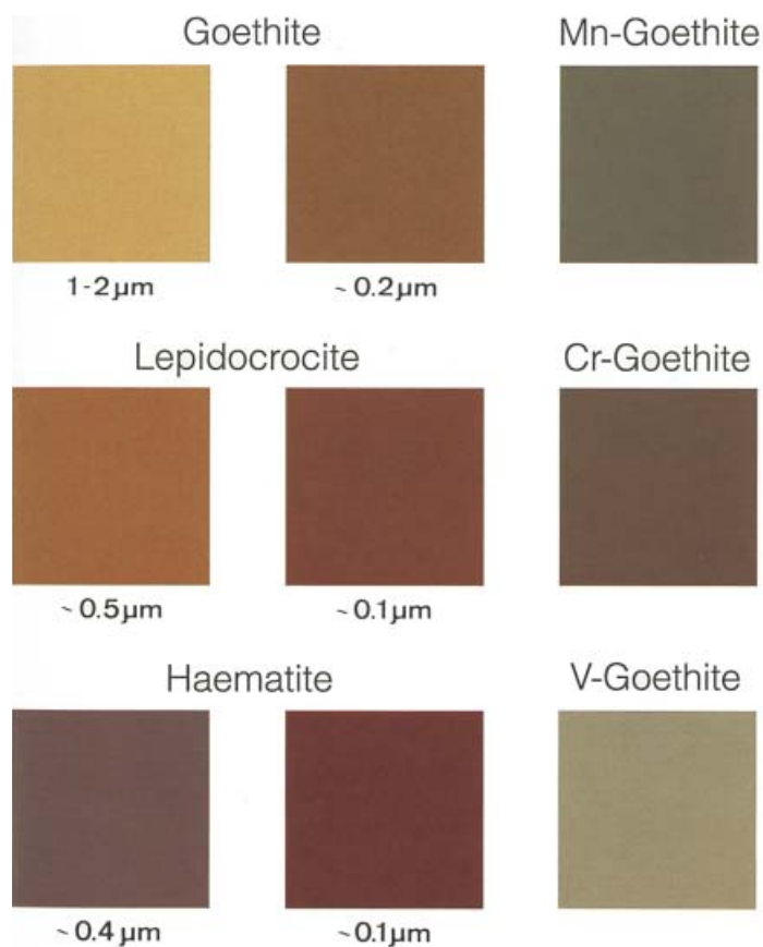
Plate 6.II Effect of particle size and cation substitution on the colour of \text{Fe}^{\text{III}} oxides
