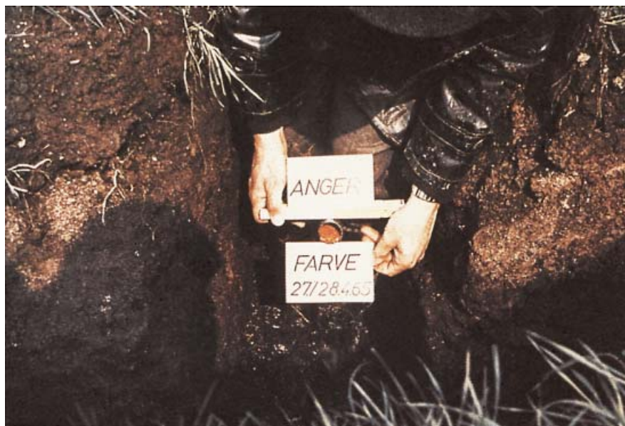
Plate 15.V Drain pipe clogged with ferrihydrite (courtesy H. Kuntze).
