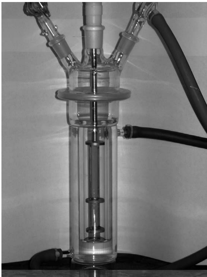
Fig. 1.3 Small scale oscillatory baffled reactor (OBR) for gram scale suspension polymerization.
