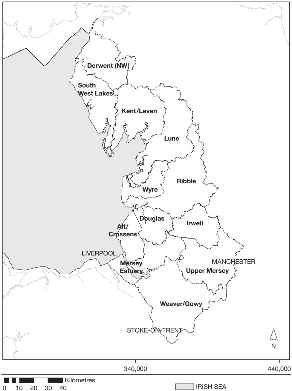
Fig. 1.3 The north-west of England showing the land surface made up from abutting river catchments. The world's entire land surface is divided up in this way. Many catchments adjoin those of a larger river and eventually discharge to the seas and oceans, but this is not necessary. Many catchments are entirely land-bound and water leaves them, not at an estuary, but by evaporation to the atmosphere.
