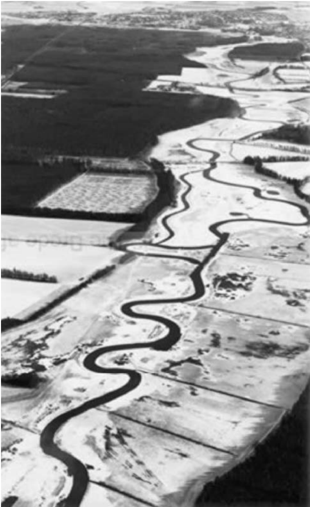
Fig. 1.7 The River Brede in southern Denmark was previously greatly modified by straightening and deepening to more efficiently drain surrounding agricultural land. Recently parts have been restored to their former course and the floodplain re-established. Segments of the original straightened channel can be seen along with the restored meanders, side channels and floodplain.
