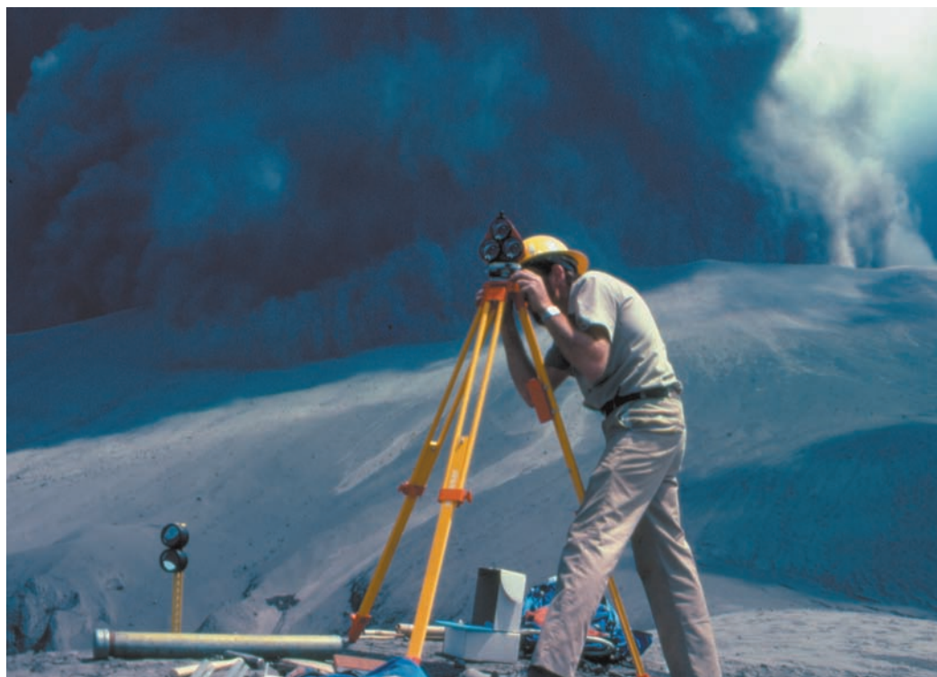
Fig. 1.8 EDM reflector at Pasir Bentang station below the erupting crater of Galunggung, August 1982. A small pyroclastic flow is beginning to cascade down the crater wall, and the thin deposits left by similar small flows are seen behind the reflector tripod. Note the permanent reflector mounted on stake to left. Photo by Dedy Mulyadi.
