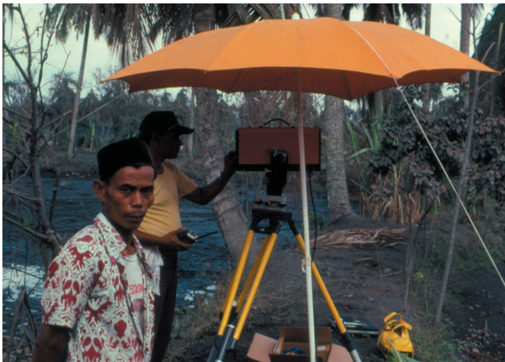
Fig. 1.5 Monitoring inflation of Galunggung volcano between eruptions by EDM from Cikasah station, 6 km from the rim of crater, where volcanologists have set up a temporary laser reflector. USGS photo by J. P. Lockwood.
