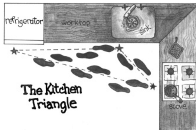
Figure 1-1: An efficient kitchen triangle.
