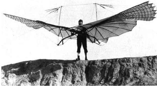
Figure 1.1 Lilienthal Glider circa 1880s showing bird influence. Reproduced by permission of Archives Otto-Lilienthal Museum
