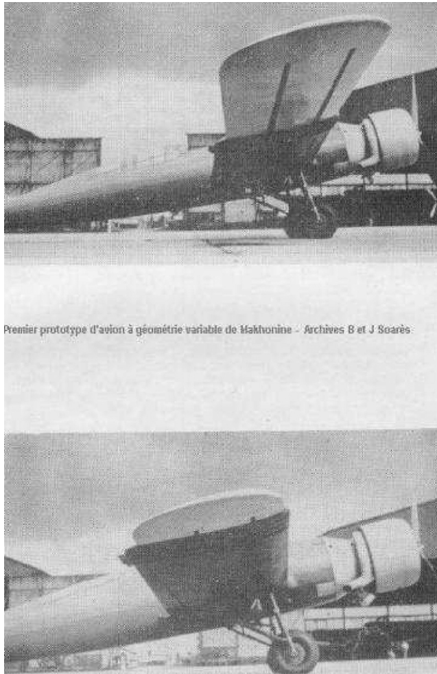
Figure 1.5 The Makhonine MAK-101 telescoping wing airplane of 1933: wing tip extended (top) and retracted (bottom)
