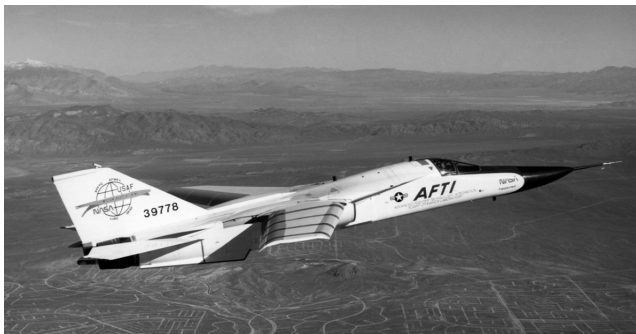
Figure 1.10 NASA AFTI F-111 Mission Adaptive Wing. Reproduced by permission of National Aeronautics and Space Administration
