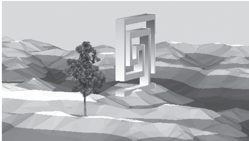
Multipatch (true 3D) features can handle multiple z values per x,y vertex, permitting realistic representations of features that include overhangs or textures
