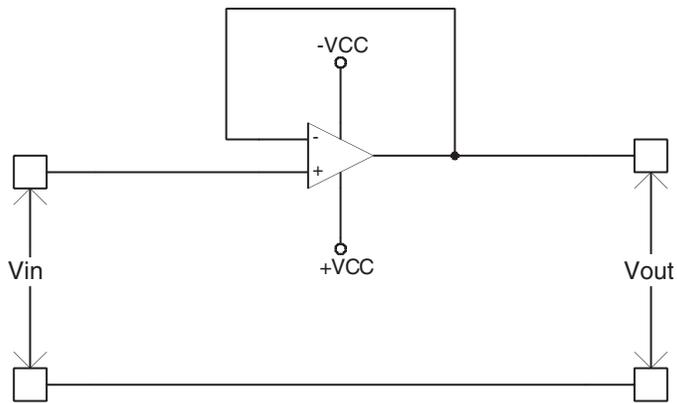
**Figure 1.6** A unity-gain buffer is a special case of the noninverting voltage amplifier in which the resistance ratio is  $R_f/R_{in} = 0$ , which translates into unity gain. This configuration is often used in biomedical instrumentation to buffer a high-impedance signal source.
