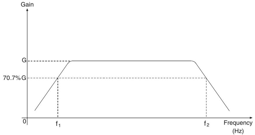
**Figure 1.1** Frequency response of a biopotential amplifier.
