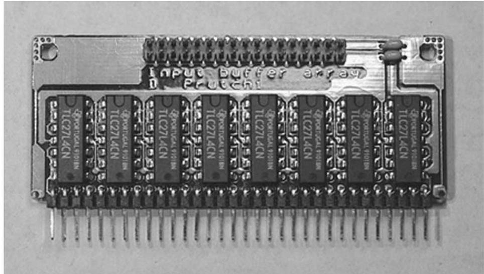
**Figure 1.8** Printed circuit board for a high-input-impedance buffer array. The output of each channel is used to drive guard rings which form low-impedance isopotential barriers that shield all input paths from leakage currents.
