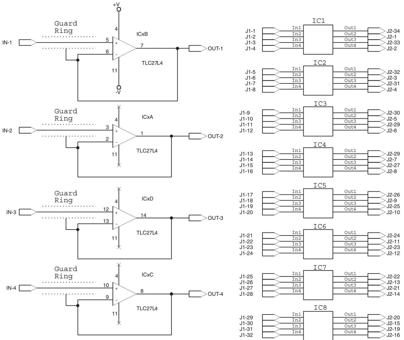
**Figure 1.7** CMOS-input unity-gain buffers are often placed in close proximity to high-impedance electrodes to provide impedance conversion, making it possible to transmit the signal over relatively long distances without picking up noise, despite the fact that the contact impedance of the electrodes may range into the thousands of megohms.
