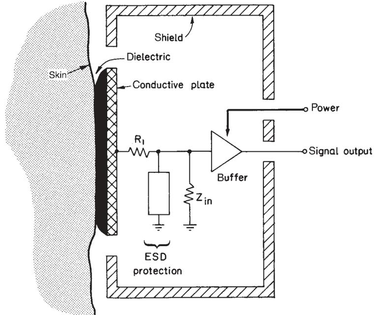
**Figure 1.10** Block diagram of a typical capacitive active bioelectrode. A highly dielectric material is used to form a capacitive interface between the skin and a conductive plate electrode. Signals presented to the buffer stage result from capacitive coupling of biopotentials to the network formed by series resistor  $R_1$  and the input impedance  $Z_{in}$  of the buffer amplifier. (Reprinted from Prutchi and Sagi-Dolev [1993], with permission from the Aerospace Medical Association.)
