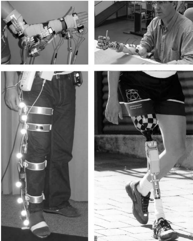
Figure 1.1 Wearable robots: (top left) an upper limb orthotic exoskeleton; (top right) an upper limb prosthetic robot; (bottom left) a lower limb orthotic exoskeleton; (bottom right) a lower limb prosthetic robot
