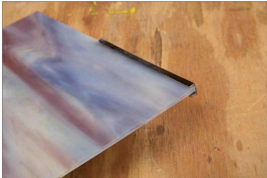
Figure 1-1: Lead came shaped into a U profile goes around the perimeter of a glass panel.
