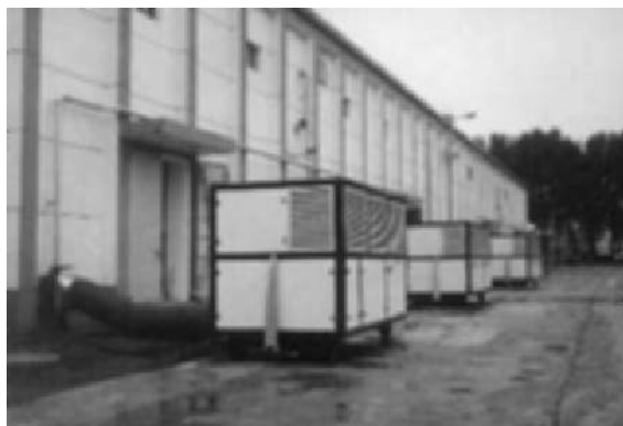
Fig. 1.3 Cereal cooler used for cooling paddy or milled rice stocks, shown here attached to a sealed warehouse in China.
