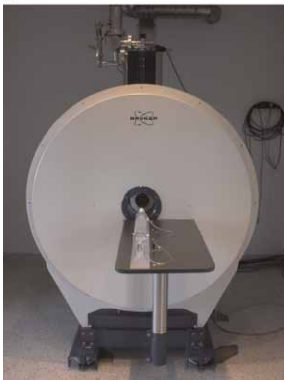
Figure 1.1.2 The superconductive magnet used for NMR experiments. (a) High field superconductive magnet for rats and mice NMR examination. This horizontal magnet, weighting 2 tons, delivers a magnetic field of 7 T inside a cylindrical access 30 cm wide. After installation of the shim and gradient coils, the access available for small animals is 15 cm wide. The chimney above the magnet is used for liquid helium refill. (b) Examination bed. The small animal is lain inside an anaesthesia chamber. The bed is positioned at the centre of the magnet bore during the examination (Courtesy of Bruker, SA, Ettlingen, Germany)
